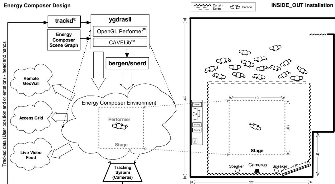
Figure 4. Component (left) and installation (right) diagrams
